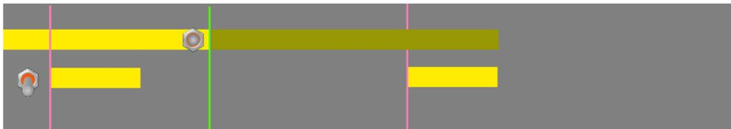
Example 9: **End Behavior = End of Skip** The solid gun will not turn off until the end of the next skip. The pattern switch may be moved into off anywhere in the gap, but the solid gun will not deactivate until the end of the next skip.
