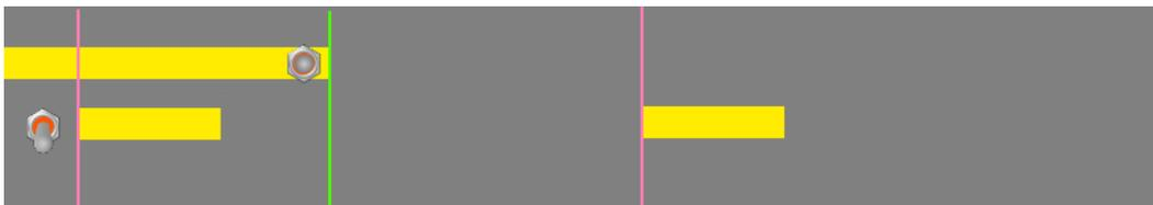
Example 7: **End Behavior = Immediate** Regardless of active skip cycle, the solid gun will turn off immediately with the pattern switch position change.
