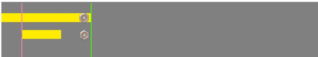
Example 11: **End Behavior = Immediate** The solid gun will turn off immediately with the pattern switch position change.
