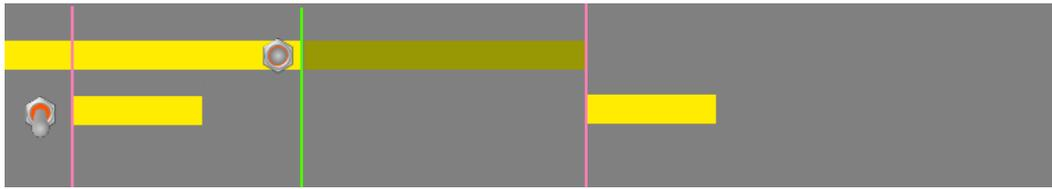
Example 8: **End Behavior = Start of Skip** The solid gun will not turn off until the start of next skip. The pattern switch may be moved into off anywhere in the gap, but the solid gun will not deactivate until the start of the next skip.
