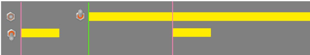
Example 2: **Start Behavior = Immediate** Regardless of skip cycle, the solid gun will come on immediately with the pattern switch change.
