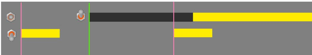
Example 5: **Start Behavior = Middle of Skip** The solid gun will not turn on until the middle of the next skip. The pattern switch may be moved into solid anywhere in the gap, but the solid gun will not activate until the middle of the next skip.
