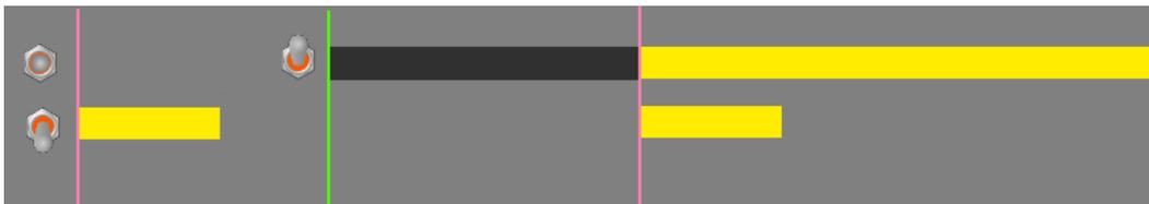
Example 3: **Start Behavior = Start of Skip** The solid gun will not turn on until the start of next skip. The pattern switch may be moved into solid anywhere in the gap, but the solid gun will not activate until the start of the next skip.
