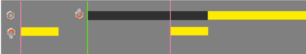
Example 4: **Start Behavior = End of Skip** The solid gun will not turn on until the end of the next skip. The pattern switch may be moved into solid anywhere in the gap, but the solid gun will not activate until the end of the next skip.
