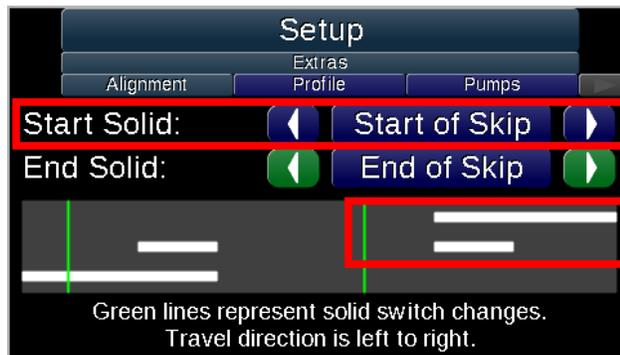
In this example, start behavior is set to end of skip. Even though the gun switch was moved to solid at the green line, it will not turn on until the end of the next skip.
