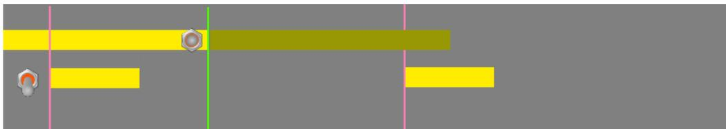
Example 10: **End Behavior = Middle of Skip** The solid gun will not turn off until the middle of the next skip. The pattern switch may be moved into off anywhere in the gap, but the solid gun will not deactivate until the middle of the next skip.
