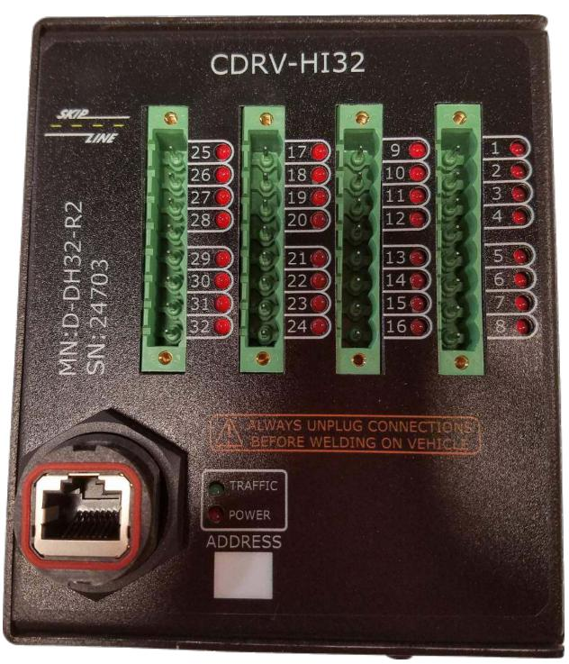
Each pin on the CDRV device is rated to 5 amps. Use 14-22 AWG wire for loads.
