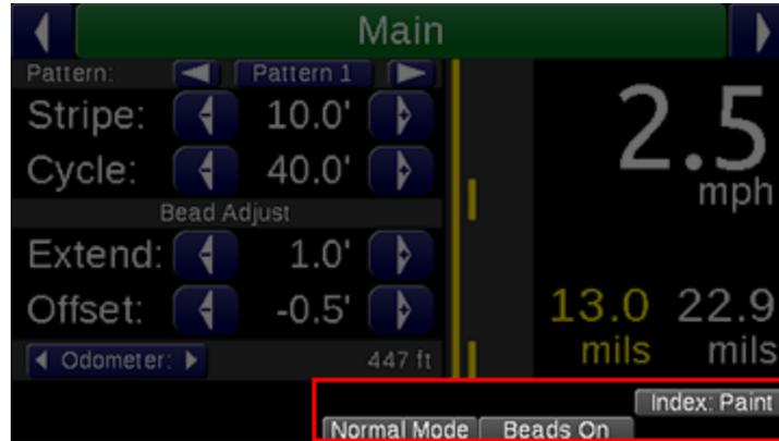
Many features can change the painted pattern. To help avoid confusion, when a setting causes a pattern change and is not indicated on the Pattern Preview, it is accounted for in the **Feature Status Indicators**. Refer to the manual section for each feature to understand these messages.
