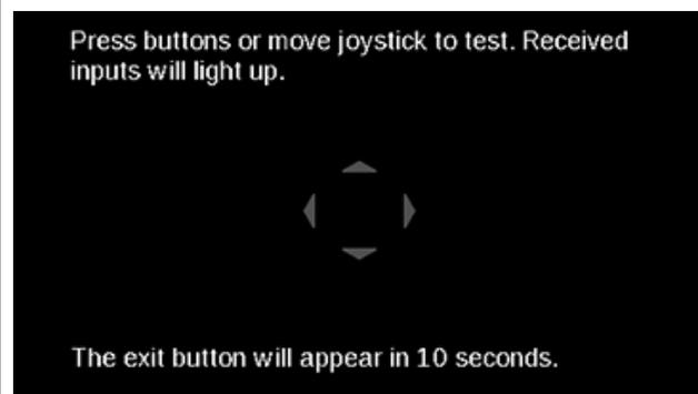
Press the navigation buttons and watch the graphic displayed on the screen. When a button is pressed, the corresponding arrow should turn green for the duration of the press and return to gray when it is released.
