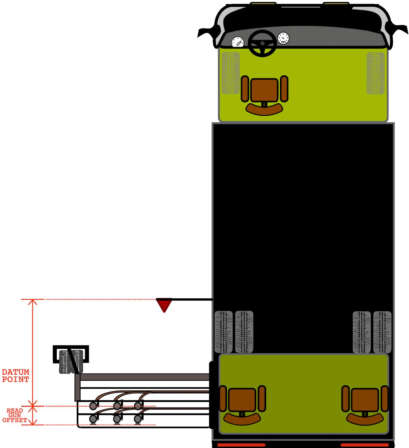
Enter the measured Datum Length distance (see 4.5.1, "Datum") and then enable Datum Point usage in the Quick Setup menu to engage this feature.
