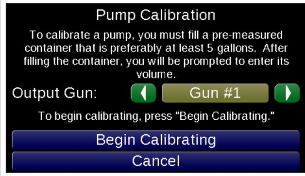
Once the pre-measured container is under the selected gun, press **Start Paint** to begin the calibration. The button will change to **Stop Paint**.
