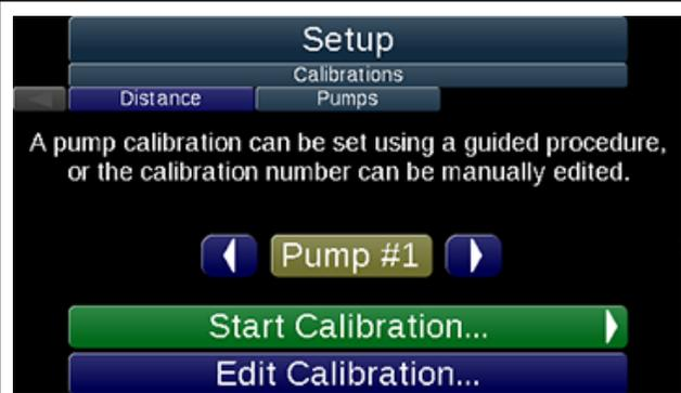
Select a gun to use for the calibration. Only select a gun that is plumbed to the pump you are calibrating. Place a container with known volume under this gun. Lower pump pressure and disable any atomizers to minimize overspray. Select
