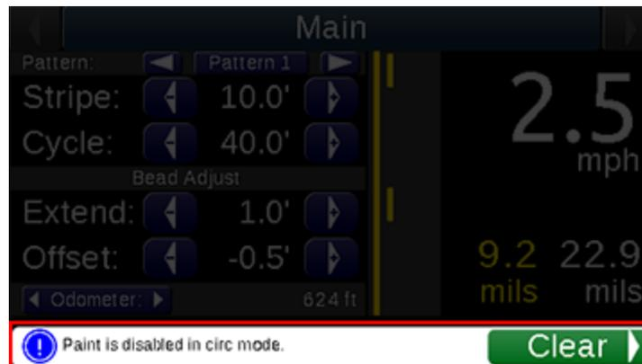
The menu provides a **descriptive alert system** to assist with understanding current activity, warnings, and critical errors that need attention. The **Information System** messages cover the status indicator area.
