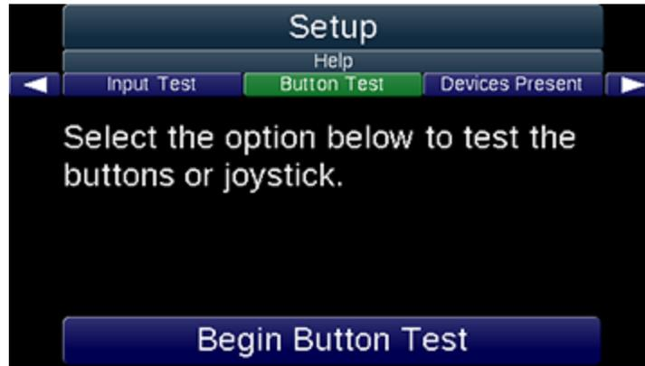
To troubleshoot issues with buttons, a **Button Test** is included in the Help options of the box's Setup menu (it also tests the Joystick if there is one). This is a quick and responsive way to check if there is an issue with the buttons.
