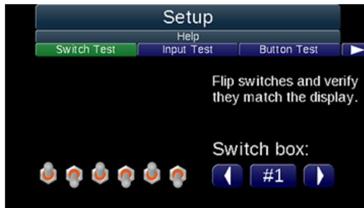
Switch failures are a common cause of difficult-to-identify operational issues. Use the Switch Test to detect malfunctioning switches.
