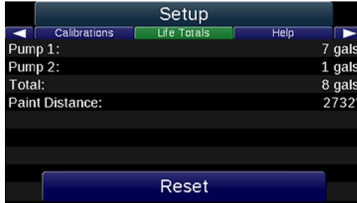
**Life totals** provide a total number of painted distance and gallons pumped. This number survives counter channel resets. The primary purpose of Life Totals is to assist the operator in knowing when to service pumps and other equipment.
