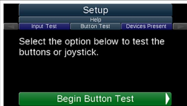
Once the **Button Test** begins, a countdown of 10 seconds will be displayed at the bottom of the screen. At the end of the countdown, the **exit** button will appear and you will be able to exit the Button Test.
