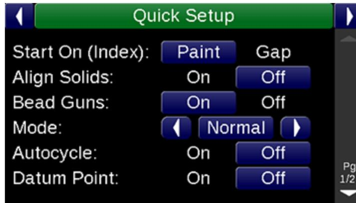
The **Quick Setup** menu provides quick access to enable or disable many features that may be used during day-to-day operations.
