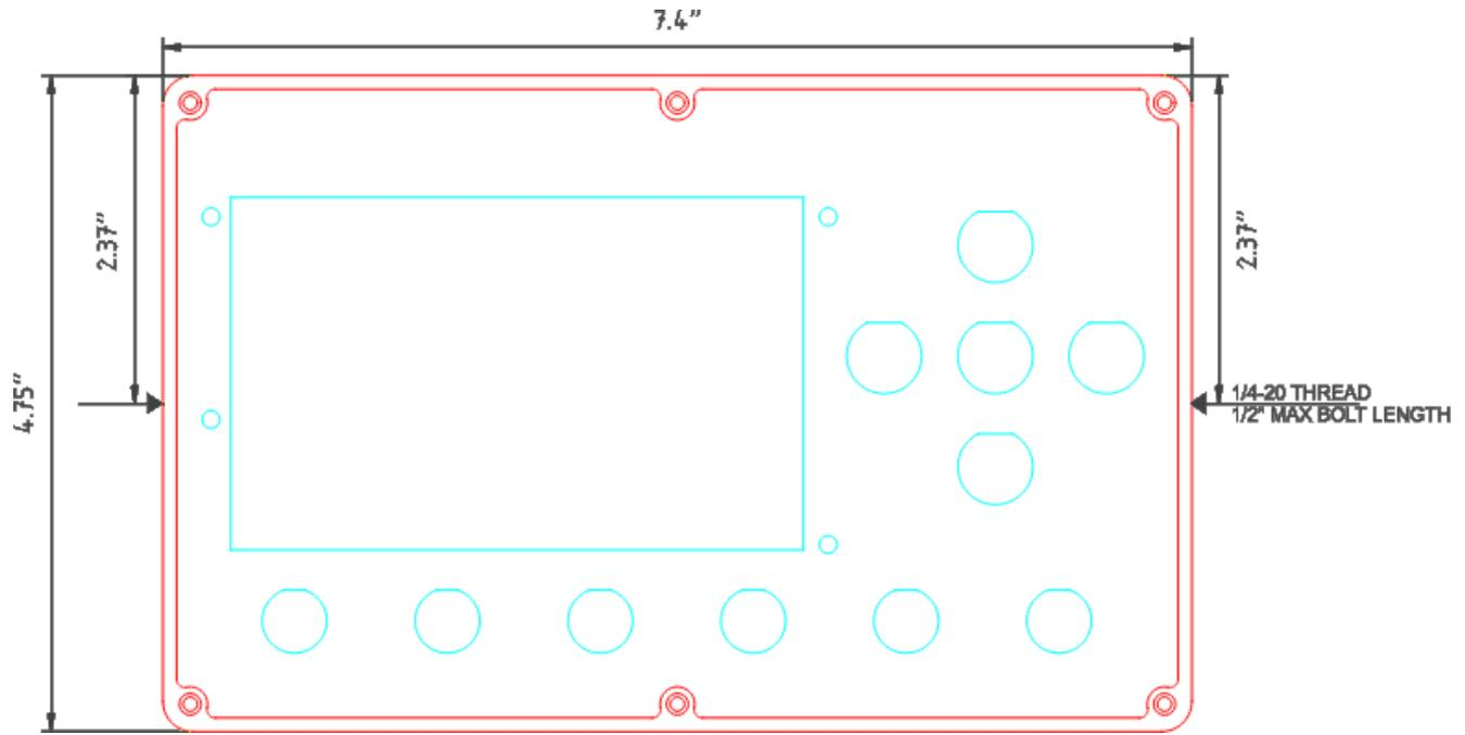
The bolt mount option is the most popular mounting option, and is used to install the MST-14 into a bracket mount or waterproof enclosure.
