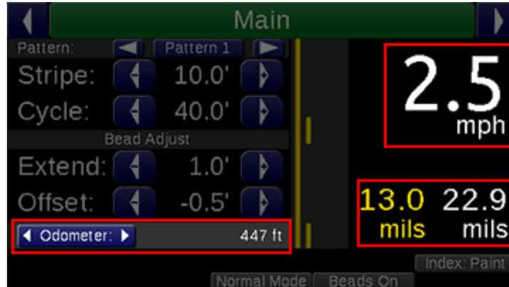
Speed is shown in large, high contrast digits for easy operator viewing.
