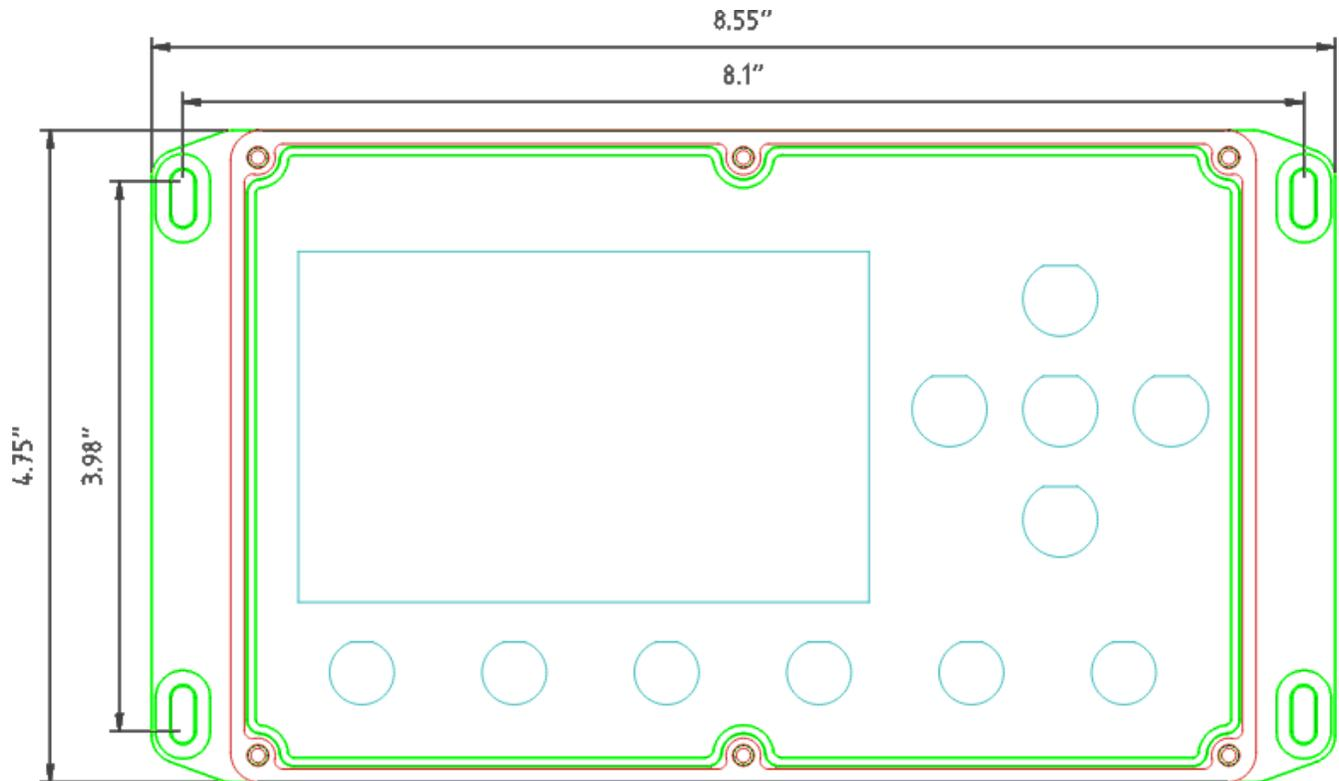
The flange mounting method allows mounting directly to a surface. The slot mounting holes fit a #8 screw size.
