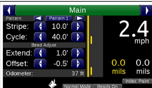
While in the Motion Demo Mode you will be able to view a simulation of the truck in motion. This includes **Counter Channels**. Motion mode will not track simulated pumpstrokes.
