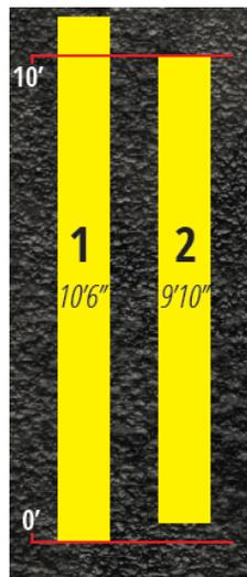
If the desired line length is ten feet, then in the above example the line marked 1 is 10'6"—six inches too long (ending late)—and the line marked as 2 is 9'10"—two inches too short (starting late). To solve the delay, use the following equation:
