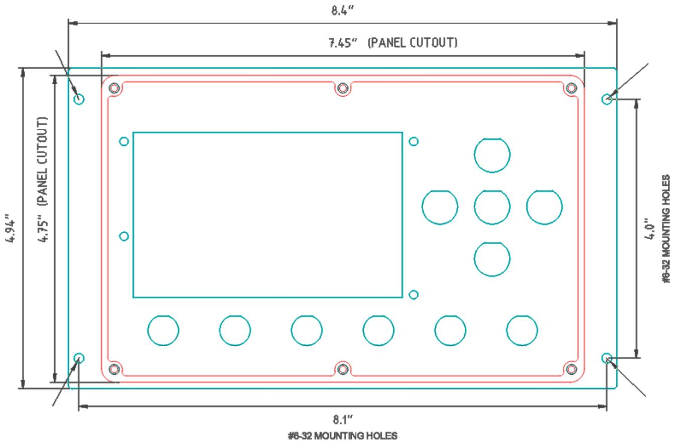
The flush mounting option was designed to allow the enclosure to mount into a sealed enclosure or console.
