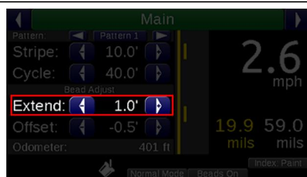
**Bead Offset** shifts the entire length of the **bead stripe**, to assist with bead coverage. This is particularly useful for dealing with shifting head and tail winds.
