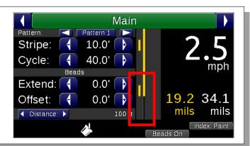
The dark yellow line indicates that the gun is not in solid anymore, but it is waiting to turn off. In this example, the solid will end aligned to the end of the skip.
